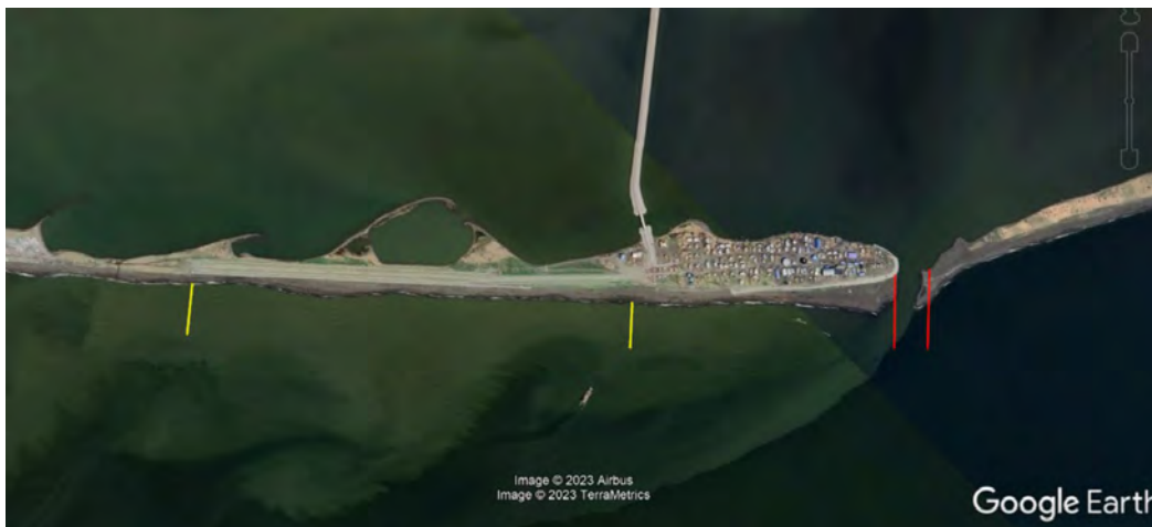
Figure 34. Alternative 4: Groins (yellow) for beach stability and jetties (red) for inlet stability
