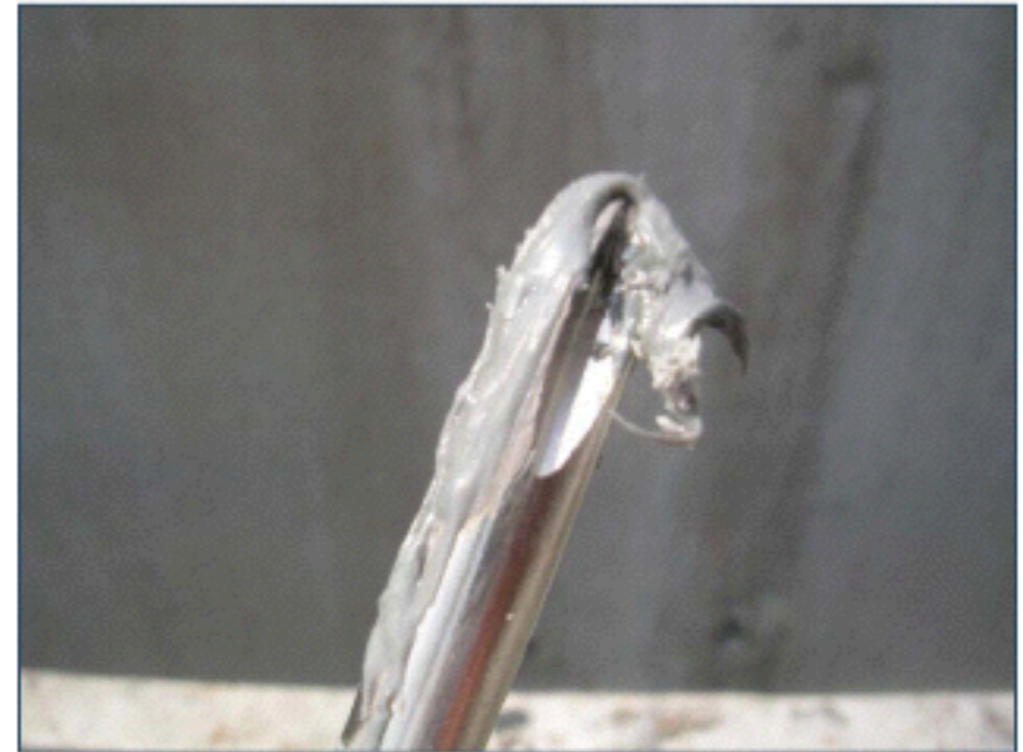
Wet epoxy component extracted from inside hole 56B
