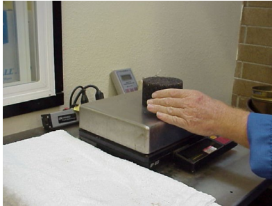
Determining mass of SSD specimen
