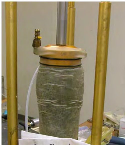
Figure 9.6 Undrained-Unconfined Compression Testing of Fairbanks Silt with Geofibers
