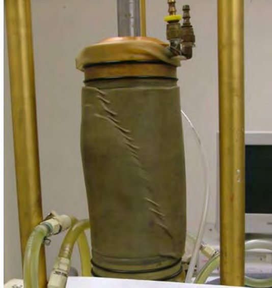
Figure 9.5 Undrained-Unconfined Compression Test of Silt without Fiber
