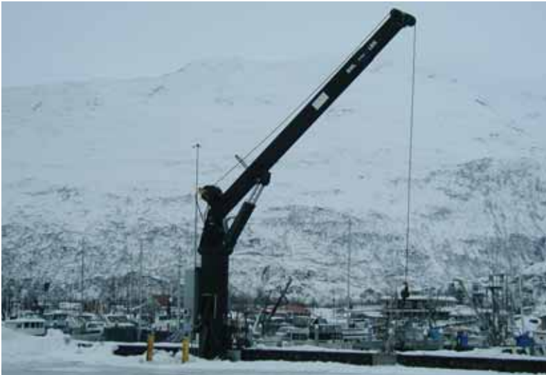
Dock-mounted crane, often referred to as a “hoist.” Cranes are used to move cargo to and from vessels.
